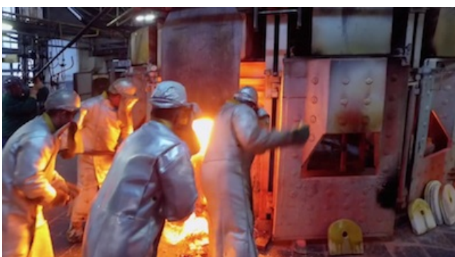
Lalique glass-blowers during the "changing of the pot" process
