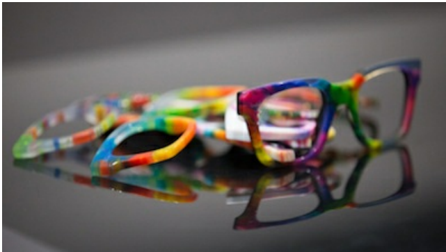
Safilo prototypes created using a 3D printer
