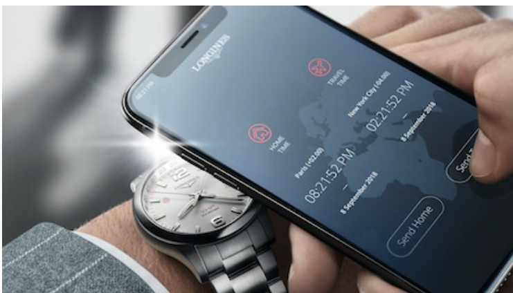
The Conquest V.H.P. GMT uses a smartphone app to set the time. Image credit: Longines
