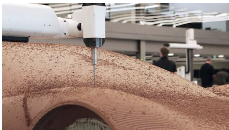
Jaguar clay modeling. Image courtesy of Jaguar Land Rover
