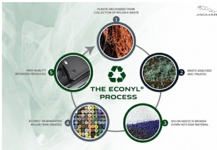
A virtuous cycle: The Econyl process. Image courtesy of Jaguar Land Rover, Aquafil
