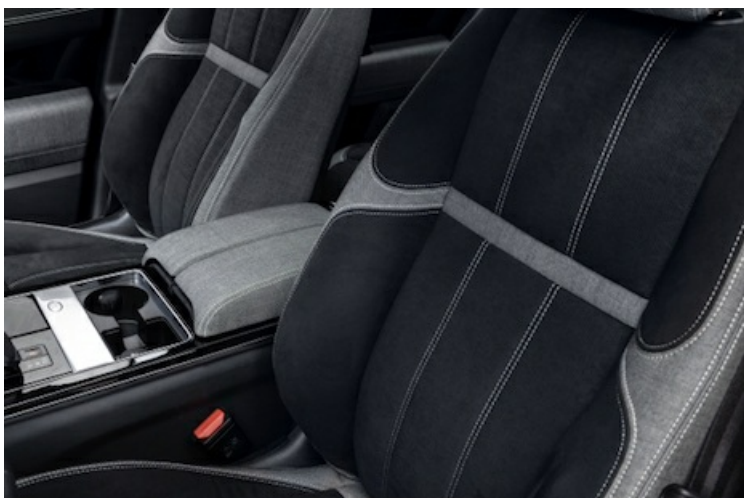
Range Rover Velar Interior made with Kvadrat, a material partly sourced from recycled plastic bottles. Image courtesy of Jaguar Land Rover
