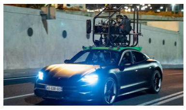
The creation of a pod car allowed a stunt driver to drive the vehicle while the actors performed inside. Image credit: Rico Torres for Lionsgate
