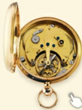
• TOURBILLON No. 1188. Sold in 1808. The back of the movement shows the tourbillon carriage and the balance. Breguet Museum collection.
